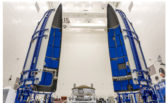
Perseverance is prepared for encapsulation in the ULA Atlas V payload fairing in the PHSF.
